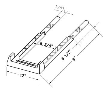
NOTE: STEPS TO BE PLACED 14" TO 16" C.C. STEPS SHALL HAVE GRADE 60 3/8" DEFORMED STEEL REINFORCING ROD CENTER.
