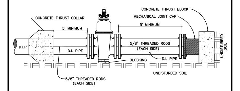
NOTE: THIS DETAIL SHALL APPLY ONLY TO TEMPORARY CAPPING.
